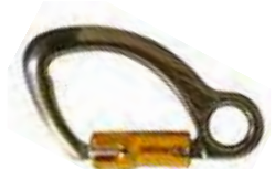
Aluminum Carabiner w/Eye 5005SAE Length: 5 1/4" (133mm), Opening: .71" (18mm), Breaking Strength: 5,732 lbs. (25.5kN)
