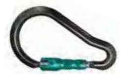
Aluminum Carabiner 5005L5 Length: 9 1/2" (241mm), Opening: 2" (63.5mm), Breaking Strength: 8,542 lbs. (38kN)
