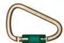
Steel Carabiner 5005I Length: 4.88" (124mm), Opening: .94" (24mm), Breaking Strength: 9,218 lbs. (41kN)
