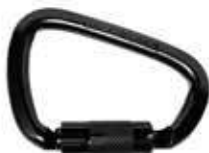
Rigging Carabiner 5005S5 Length: 4.68" (119mm), Opening: .94" (24mm), Breaking Strength: 11,240 lbs. (50kN)
