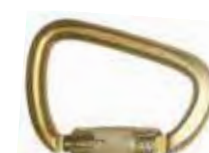
Steel Carabiner 5005S3 Length: 4.68" (119mm), Opening: .94" (24mm), Breaking Strength: 11,240 lbs (50kN)
