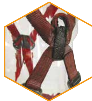
NYLON HARNESS EXPOSED TO ARC FLASH
